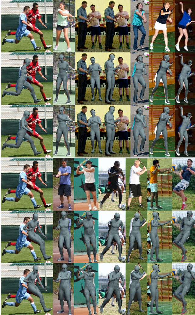
FIGURE A.14: Results of SMPLify-X fitting for the LSP dataset. For each group of images we compare two body priors; the top row shows a reference RGB image, the bottom row shows results of SMPLify with VPoser, while the middle row shows results for which VPoser is replaced with the GMM body pose prior of SMPLify [34]. To eliminate factors of variation, for this comparison we use the gender neutral SMPL-X model.
