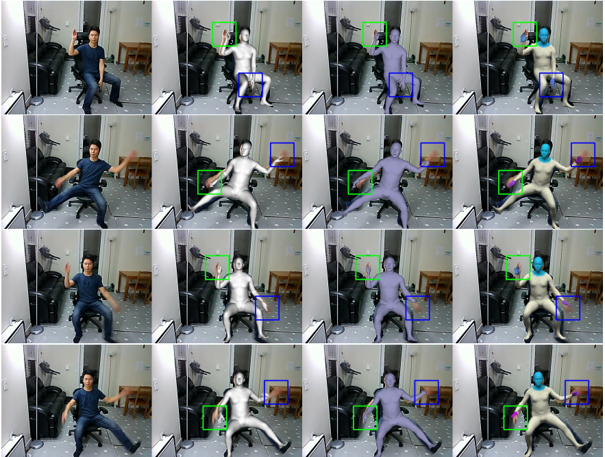
FIGURE C.3: Qualitative ExPose results and comparison to ExPose [56] and FrankMocap [295]. From left to right: (1) RGB images from video, (2) FrankMocap [295], (3) ExPose, (4) ExPose 3D body predictions with color-coded part-expert confidence. The moderator predicts the confidence of body/face/hand experts, redder means higher confidence in the body expert rather than the results from face/hand experts. Thanks to the moderators, PIXIE is more robust to low-quality part images. For example, when the hand is blurry, ExPose still predicts a plausible wrist pose, instead of an unnatural twist.
