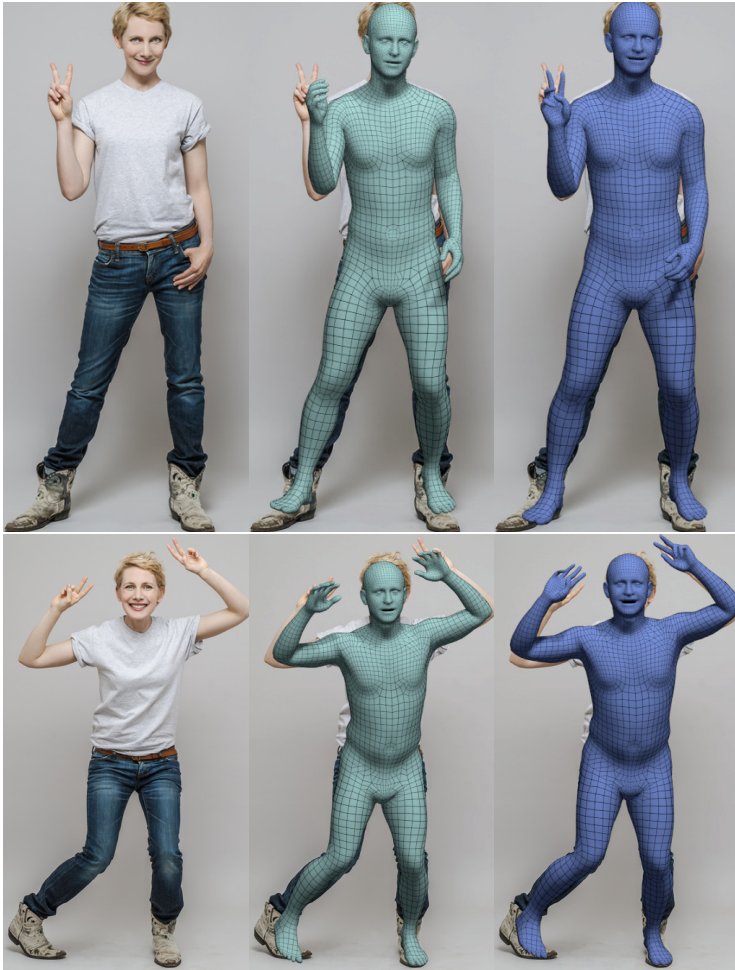
FIGURE 3.4: Left : The input image. Middle : Naive regression from a single body image fails to capture detailed finger articulation and facial expressions. Right : ExPose is able to recover these details, thanks to its attention mechanism, and produces results of similar quality as SMPLify-X, while being 200\times times faster, see Tab. 3.3.
