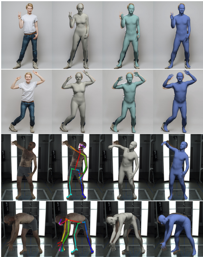
FIGURE B.8: 1. The input image, 2. OpenPose detections, 3. SMPLify-X fitting, with the neutral model and default focal length, 4. ExPose. When 2D keypoint detections are missing or wrong, optimization based methods, such as SMPLify-X are unable to avoid implausible poses. Furthermore, they heavily depend on their initialization and can produce unnatural poses and shapes, when their initialization heuristic fails. Regression methods, such as ExPose, avoid these problems and can provide better initialization points, closer to the actual solution, and accelerate convergence.
